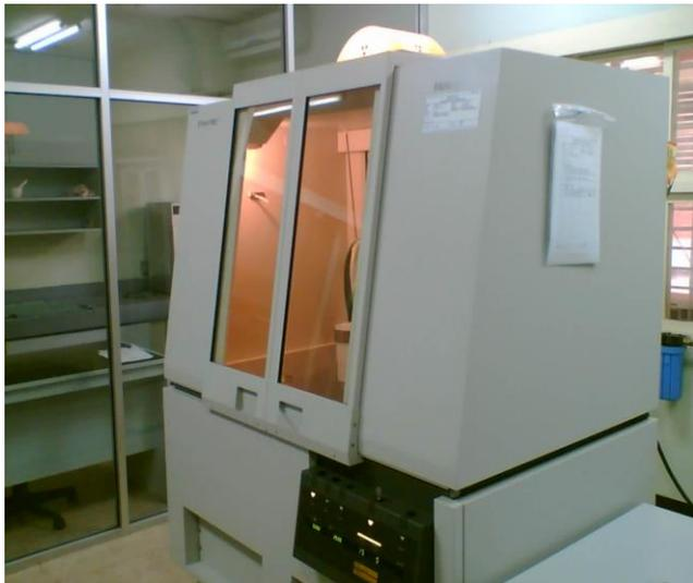
Gambar (8.27). Peralatan XRD tipe PANalytical Diffractometer.
