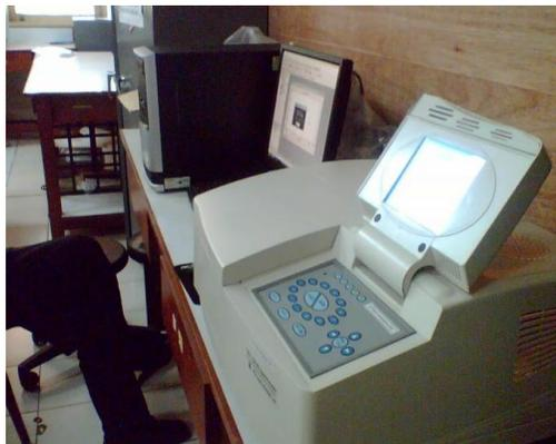
Gambar (8.22). Peralatan UV-VIS tipe PG Instruments Ltd T70+ .
